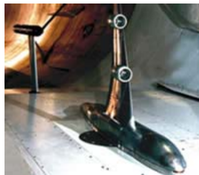
Drag Reduction Wind Tunnel Tests
